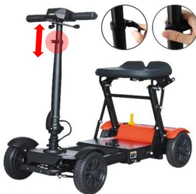
Open the handle and adjust the height of steering column to fit for you, then lock
