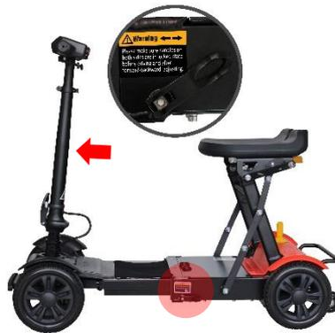
One hand hold the seat, another hand push the steering column forward, then lock both sides handles
